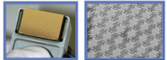
FIGURE 2. Collimator Lens Array and MEMS Element.
